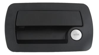
This flush mounted paddle is a redesign of our 030-0400 paddle handle for entrance doors on recreational and specialty vehicles. Containing the same proven mechanical details as previous with a modernized look, it can be used in FMVSS 206 (ECE R11) applications and features a remote pivot plate and lock cam actuation.
